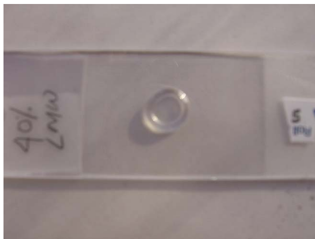
Fig. 1. A picture of the donut-shaped drop that is left behind after toluene evaporates from a solution of low-molecular weight polystyrene dissolved in toluene has been shown.
